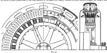
of its advantage of the single stationary exciting coil, the inductor alternator has such a high degree of leakage, and the effect of armature reaction is so detrimental in it, that the type has been gradually abandoned, and a return has been almost universally made to the heteropolar alternator with internal poles radiating outwards from a circular voke-ring. The construction of a typical machine of this class is illustrated in fig. 37.
